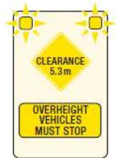
Overheight warning signs are located before both approaches to the Heysen Tunnels and work in conjunction with laser beam vehicle height detectors to detect vehicles that are too high to safely transit the tunnels.
